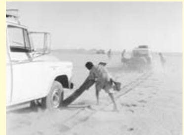
Inserting a Sand Track Under a Moving Truck
