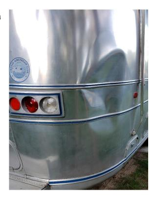
So, we removed the trim pieces (lots of rivets to drill out). I got out my new pneumatic dent puller, fired up the air compressor, hooked the dent puller up to the air compressor, put it on the dent, drew a vacuum with the air compressor which suctioned to the trailer quite well, and tried a small sample pull to see how hard it was going to be to remove the dent.
