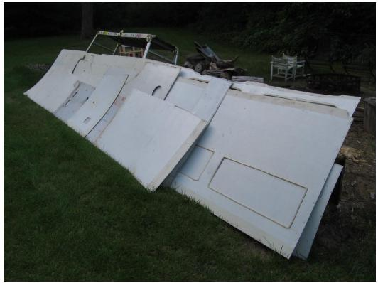
Here are all the inner skins ready to be coiled up and stored while we replace the plywood floor and make some frame repairs.
