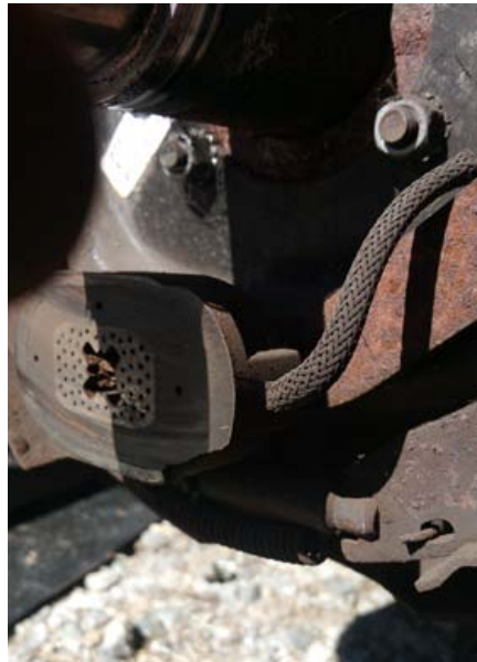
Brake magnet missing a piece out of the bottom side.
