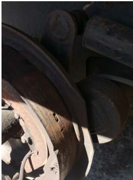
Brake assembly missing its lining material,
