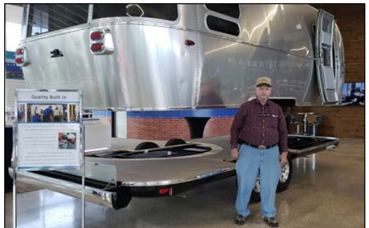
Above: NORVA President Dick Arnold stands alongside an Airstream trailer shell suspended above its chassis.
