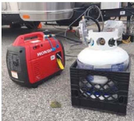
Honda EU2200i with Hutch Mountain propane conversion and adapter
