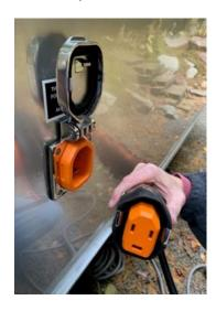
Lastly, check the trailer wiring for the correct polarity. Two amber lights and no red light on the tester and we are good to go.
