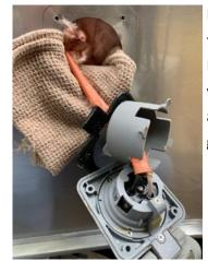
Remove the two screws from the strain relief bracket. Slide the wiring cover back to access the wire retaining screws. Notice a towel was placed over the sharp edge to protect wiring from nicks and cuts. Loosen the wire retaining screws and remove twist lock plug. Remove the cover and old rubber gasket.
