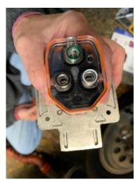
Insert the wires into the proper color terminal and tighten the wire terminals with the included allen wrench.
