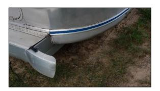
Between trips and being sick, I have been able to straighten it out about 98% of the way and brazed the cracks back together.
