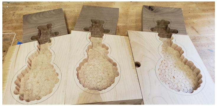
These are the bowls with the centers roughed out using a  $1\frac{1}{4}$ " forstner bit. The pencil lines show the outline of the template I bought and use with a router to shape the insides of the bowls.
