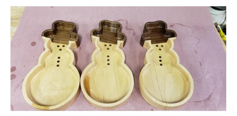
Here's the three bowls finished. To my dismay, the bowl on the right has a crack in the maple that went all the way through the wood. However, I filled the crack with CA glue (super glue), and it's all solid now. I tend to celebrate wood defects and not try to cover them up in my wood working. Two bowls are presents and one is for us.
