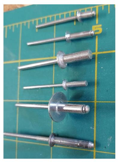
Here are the ends of the rivets. You can see that the two closed end rivets have a solid bottom so water will not leak through them.
