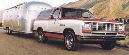
5,000 LB. MAXIMUM TOWING CAPACITY. optional. For towing jobs, both Ramcharger Two and the 4WD Ramcharger mate a heavy 5.2 liter V-6, which delivers 143 horsepower and 250 foot-pounds of torque, with a 3-speed automatic transmission. All standard equipment. Drive smart. Buckle up for safety.
