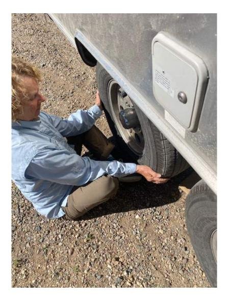
TIGHTEN lug nuts on opposing sides of the pattern 12 o'clock, 6 o'clock,
