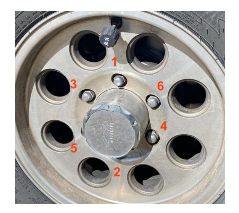
Torque your lug nuts to 110 foot pounds with the torque wrench. Retorque after 50-100 miles.
