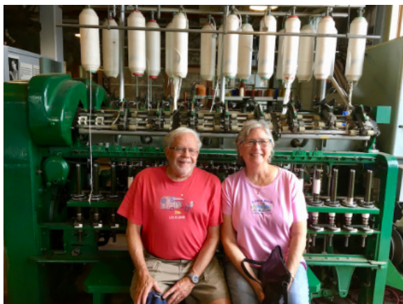
Bard & Kathy in front of a spinning frame machine that pulls and twists cotton fibers into threads.
