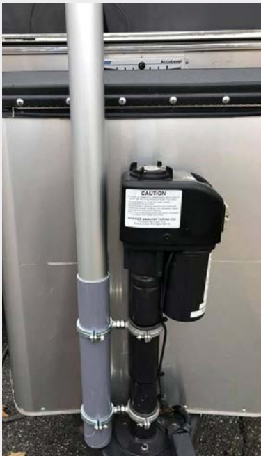
9. This is how we installed the extendable flag pole to our Airstream jack using pairs of clamps connected by stainless steel rods. This is very efficient way to mount the antenna and can be installed or repacked within three minutes
