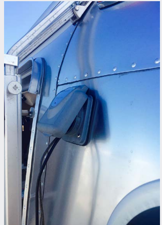
8. Cables to the Dishy antenna run through a modified Furrion shore-power port that we installed adjacent to the main door. We installed the cable port some years ago to be used for cables from the cellular booster and for the Wi-Fi booster antenna
