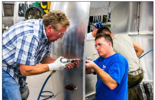
*There are many different kinds of modern rivets. The rivets that attach the aluminum panels of an Airstream body together are called buck rivets, named after the "bucking" process that shapes the head.*
