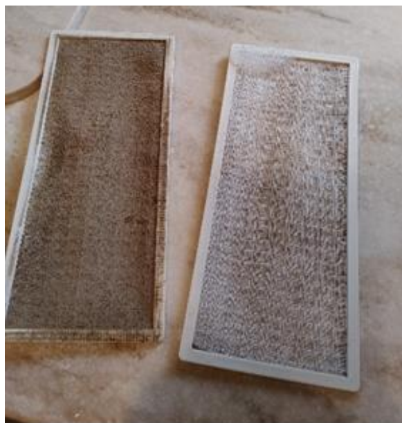
Inside screen filters: before and after cleaning
