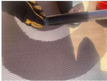
The end of the torque wrench is the "dial" that is used to set the foot pounds.
