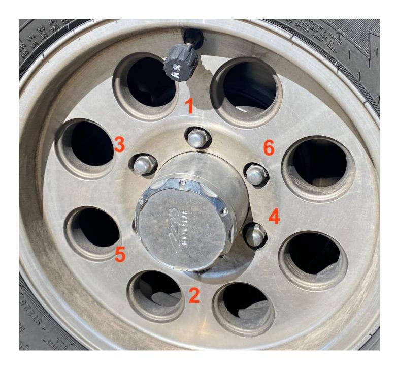
Torque your lug nuts to 110 foot pounds with the torque wrench. Re-torque after 50-100 miles. When storing the torque wrench reset it to "0" foot pounds.
