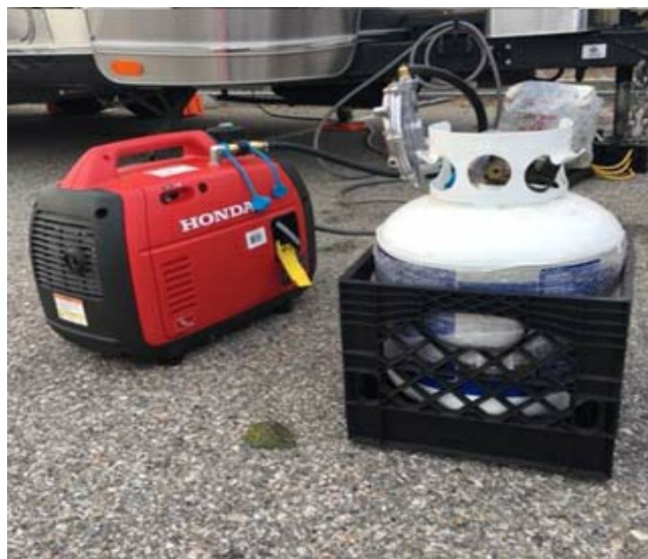
Honda EU2200i with Hutch Mountain propane conversion and adapter attached to external propane canister during Rose Parade Rally. With additional connections, it can be also be attached to the trailer's tanks.
