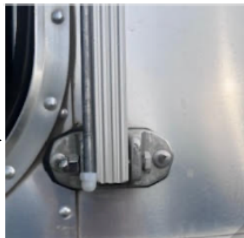
Rod re-installed with threaded end & new plastic nut tip.
