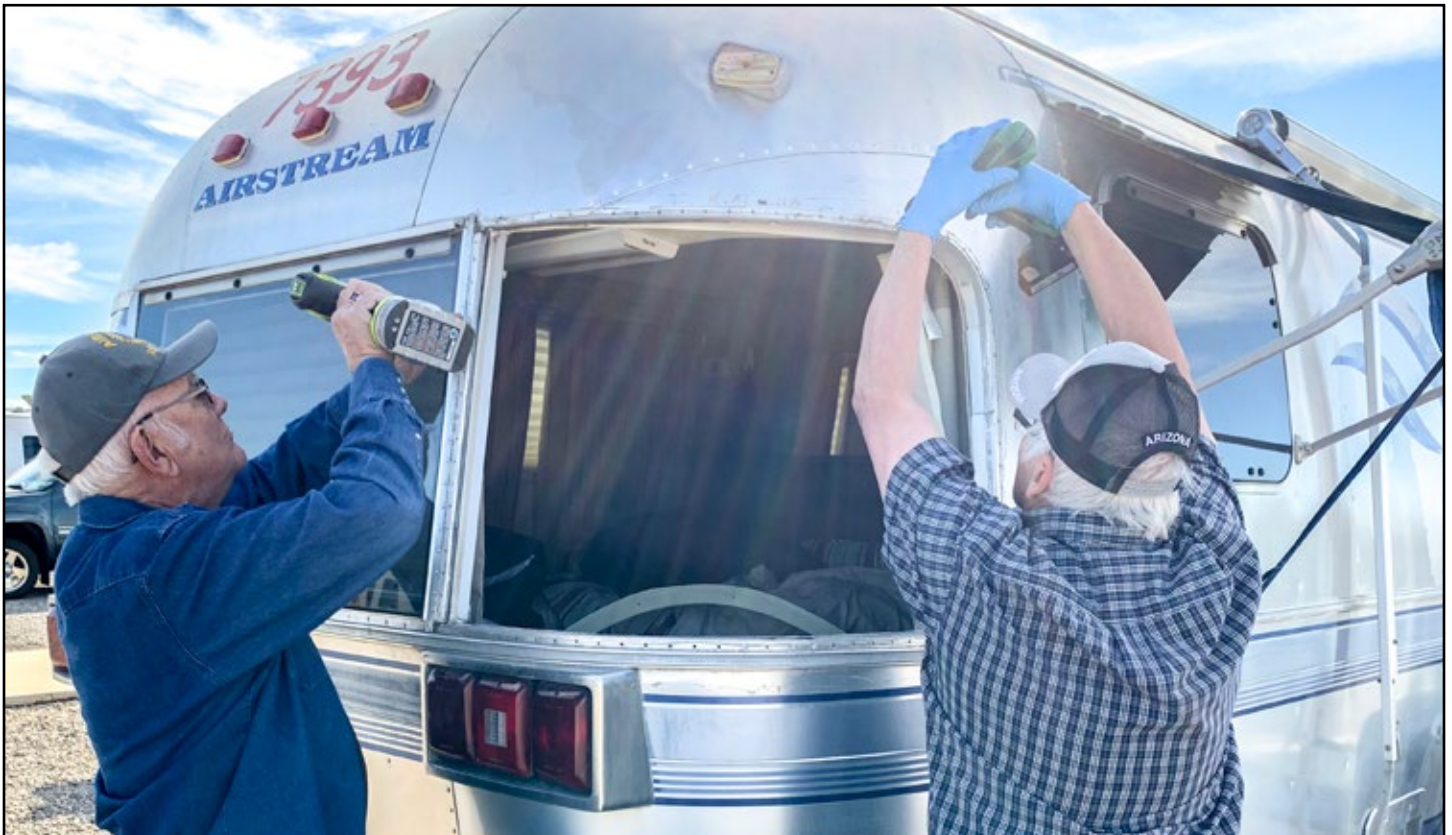
John Fikkert and Ron Larson replacing a curved window in an Airstream!
