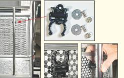
Step Brace Clip - The clip is designed to be used for transit only. For both the front and rear door models, mount the step brace clip approximately 5-1/2" from the side and 1-3/4" from the top of the screen guard on the hinge side of the door. Mount the clip so it folds up when not in use. All stainless steel hardware is included.
