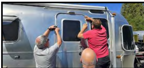
Fixing a very loose door hinge
