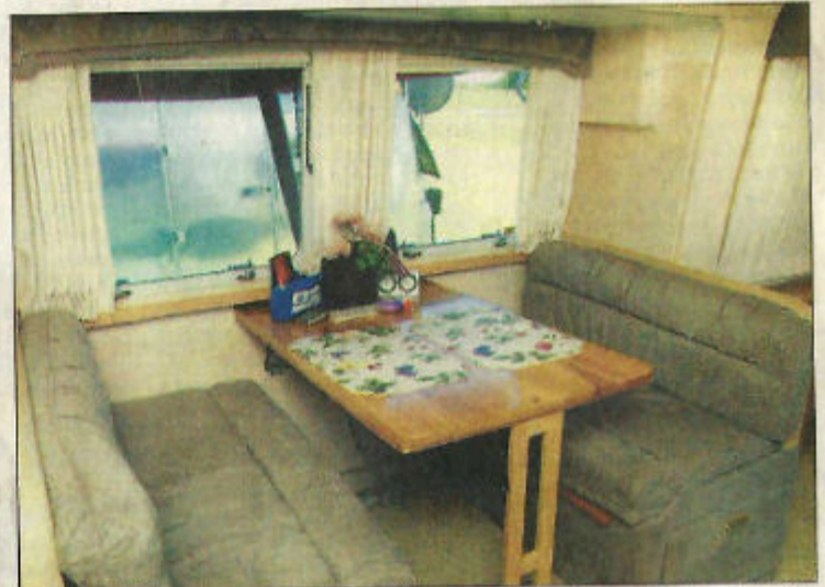
The dinette slides in and out of the Airstream to allow for smooth travel while on the road and more living space when parked.
