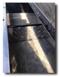
I had pre-drilled holes in the angle piece and was only able to get the drill in from the top to drill two of the four holes I had pre-drilled. This was enough as you can temporarily use blots to bolt the divider underneath the bumper trunk
