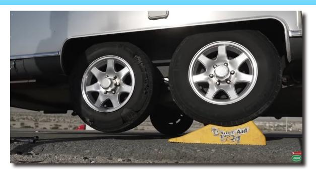
Here's a tip if you have a double or triple axle trailer. Rather than using a jack, use blocks or curved levelers; there are many varieties. It is easier (no need to find the jack or crawl under trailer), safer (as a jack is less stable), and faster. Just remember to loosen the lug nuts on the bad tire before rolling up on the good one.
