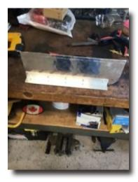
Next, I riveted a piece of one inch aluminum angle to the cutout diamond plate piece. This would allow the divider piece to be put in place and riveted to the floor of the bumper trunk. I removed the rubber mat from the bumper trunk so that I could drill some holes in the floor of the bumper trunk to attach the angle piece with the divider.
