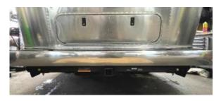
Installation was very easy on our International as the rear bumper access made it simple to drill the four mounting holes. Other trailers are a bit more difficult, but they include a snake tool that helps get the bolts in the right hole. It comes with two bumper brackets, two draw bar brackets and the draw bar with the 2" receiver. Also included are all the bolts, nuts and washers you need.
