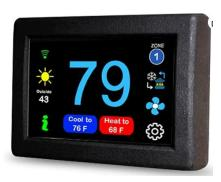
The entire install took less than 15 minutes. So what is so good about it? Well it has a very simple and easy to use interface. Once you plug it in, it is preprogrammed for your AC unit (you have to specify when ordering). So it is plug and play simple. It also has Wi-Fi and Bluetooth connectivity plus a program option if you want to set different temperature profiles.
