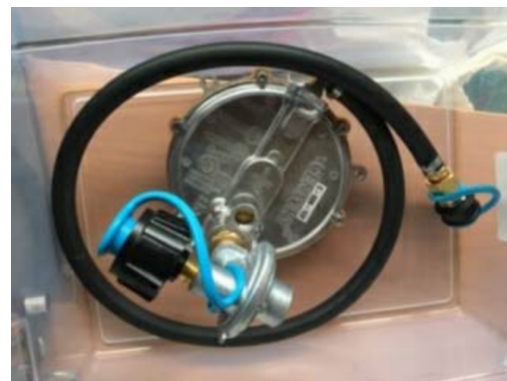
Close up of Hutch Mountain hoses and external propane regulator
