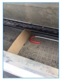
stands for Cardboard Assisted Design. First, I measured the inside of the bumper trunk and then cut a piece of cardboard to approximately that size. By fitting the cardboard in and cutting it to fit I came up with a perfect template for the interior divider.
