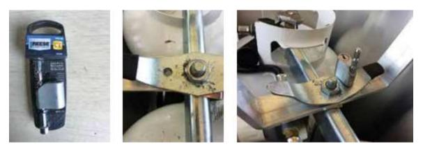
Just line up your gas bottle hold down with the bar on bottle cover and drill a <sup>1</sup>/<sub>4</sub>" hole and install coupler lock.
