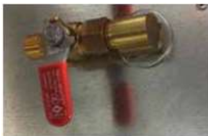
Ball valve with brass elbow (currently used on some Airstream models as a low point drain).
