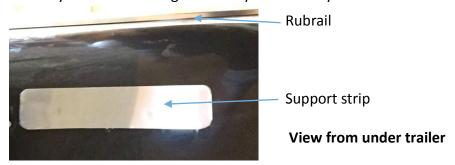
Measure the distance between the support brackets on the hose carrier tube and then mark for inboard metal support strip. You will want the tube brackets to be in the center of support strip.
