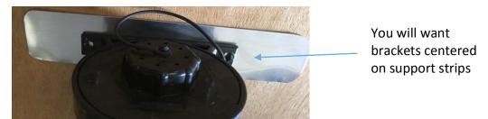
Once both support strips have been measure and in line you are ready to attach the tube. Unless you have an extra set of hands ,you will need something to support the tube while drilling. A jack stand works well for this.
