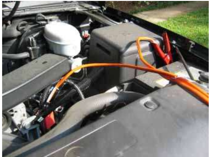
Attach the last cable clamp to an engine block ground and avoid potential sparks near explosive battery gasses.
