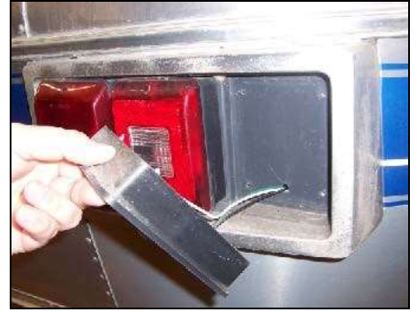
Fig. 4: Tilt from top to expose wires
