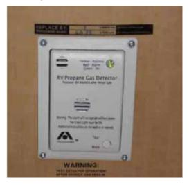
alarm cannot be silenced. An end of life label is affixed at the top of the detector to inform the customer the month and year the LP detector must be replaced. This will prevent customers from unexpected and of life alarms
