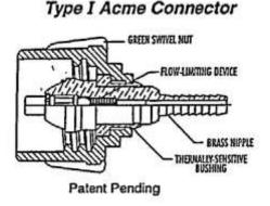
The G-1851-A03 appliance side swivel nut fitting is female 1-5/16" ACME x 1/4" MPT. As the appliance side of the Type I connection, it makes a positive connection by threading on to the ACME threads of the LP tank valve with a user-friendly right hand turn motion.
