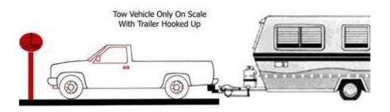
Your vehicle and trailer must be fully loaded and fueled just as they will be when you are leaving for a trip. First, drive on to the scale with all 4 wheels of the truck and record the weight of the truck with the trailer attached.
