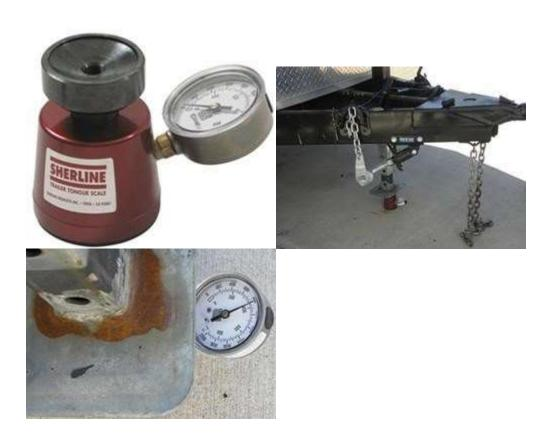
These images show the tongue weight scale in use. Be sure that the trailer is level and parked on level ground when you weigh it.
