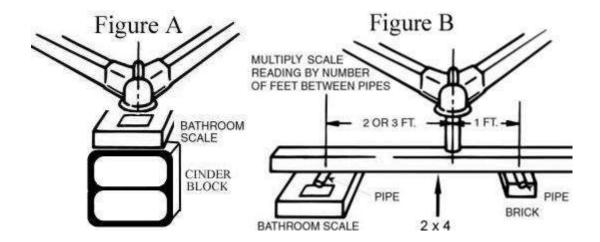
You can use a bathroom scale and a box to measure tongue weight of smaller trailers. Place the coupler of the loaded trailer on the scale at normal towing height (Figure A). For heavier tongue weights, use the second method (Figure B). Be sure to perform these measurements on a level surface and with a leveled trailer.
