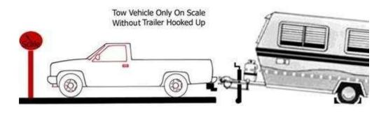
Next, unhook the trailer and jack up the trailer tongue so there is no weight on the hitch ball. Make sure that the trailer jack is not on the scale. Record the weight of only the truck on the scale. This is your gross vehicle weight (GVW). Now, subtract the GVW from the weight of the truck with the trailer attached. This will give you the tongue weight of your trailer.
