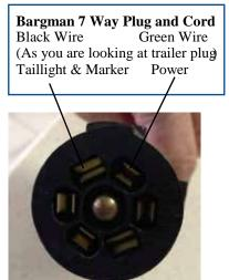
The **7 way power cord** is the critical link between your tow vehicle and your Airstream. While it is simple "plug and play" it does require some attention so brakes and exterior trailer lighting are ready to go when you are.
