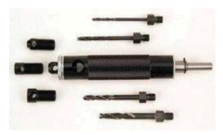
This tool allows quick and accurate removal of button head rivets and blind fasteners. Locking ring at back of tool permits depth adjustment so you only drill out rivet head. Guides and threaded drill bits are included to remove #40, #30, #21, #10 rivets. Replacement bits are available.
