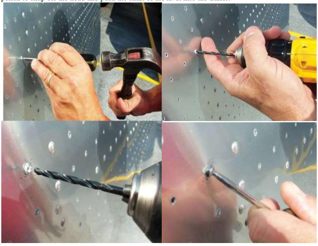
Another way to safely drill out and remove an Olympic rivet would be to use a drill guide.
