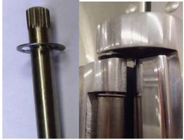
The part # for the main door hinge pin is 381552-100 & the C clip is 381552-101. This hinge pin will also work on Classic motorhome door hinges as well.
