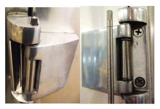
Airstream has added a groove to the hinge pin that accepts a "C" clip that is installed at the top hinge joint once the pin has been inserted into the castings.
