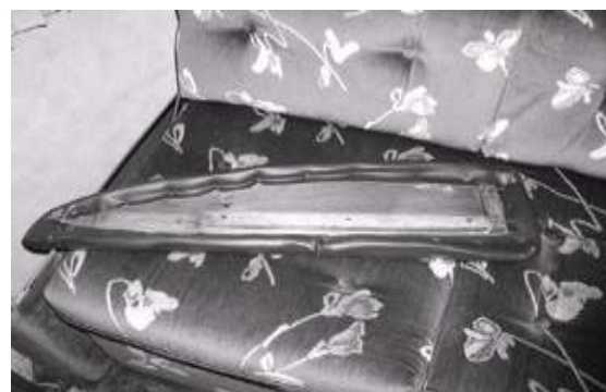
L shaped cleat on bottom of arm holds the arm in place – size and position match original factory arm.
