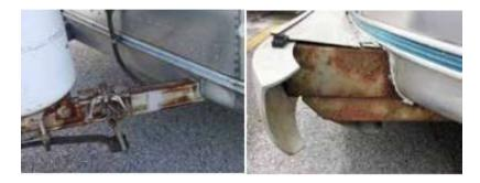
The first thing is to determine if you will be touching up a small spot or doing the complete hitch (a-frame)/frame. If you just have a small spot rusted, you can just sand and hit with some primer and then some matching paint.
