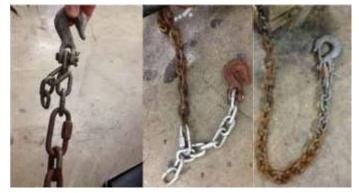
In need of some safety chains These chains all have been added on to but may only be as strong as the weakest link. Use proper rated chains, links and hooks.
