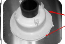
Butyl-757 should slightly ooze out of holes indicating a good seal.
